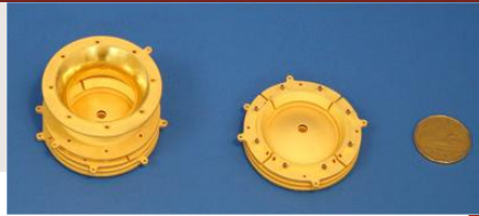
Measurement Penning trap
