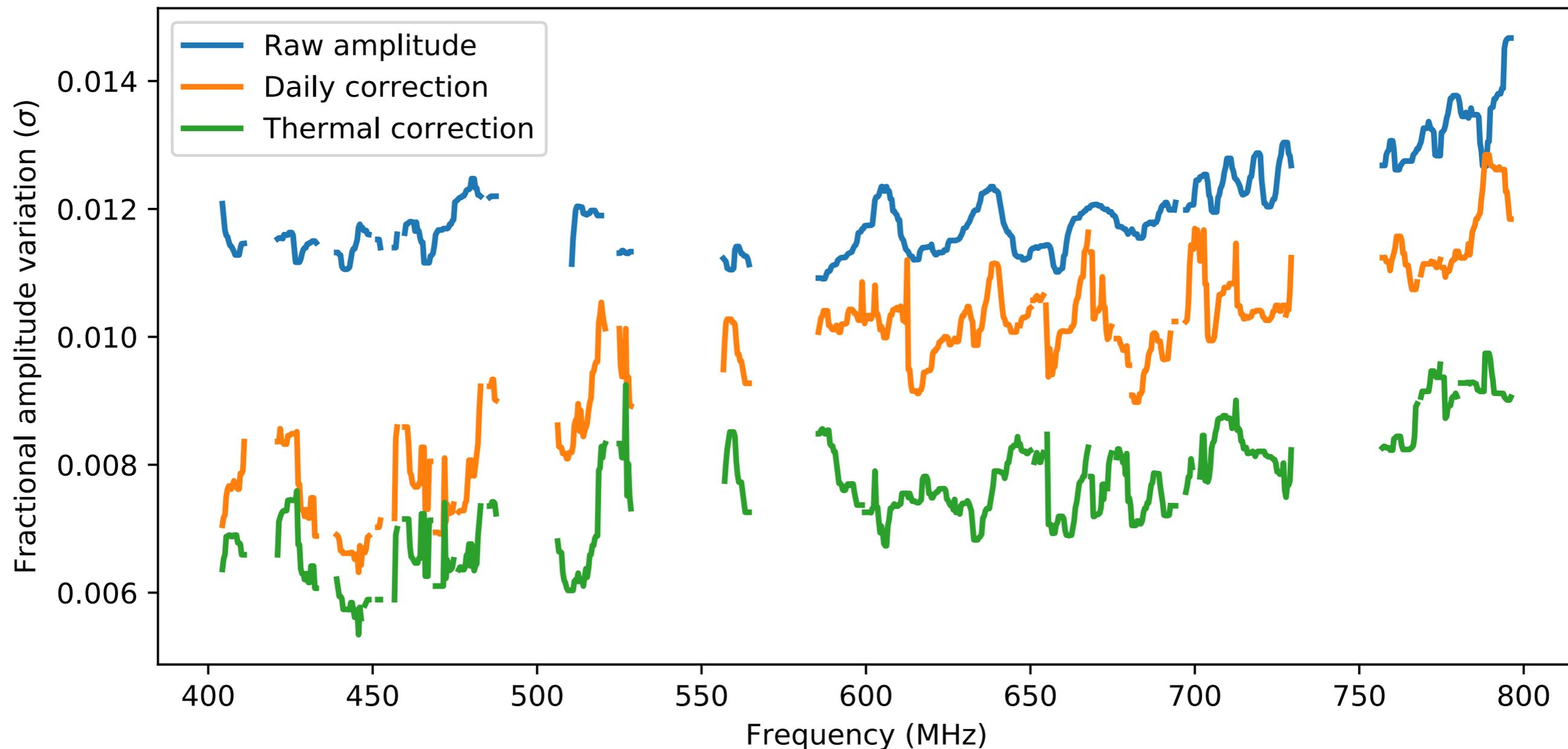
Common mode amplitude stability. **Raw**, **after daily calibration**, and **after daily calibration and correction based on outside temperature**.
