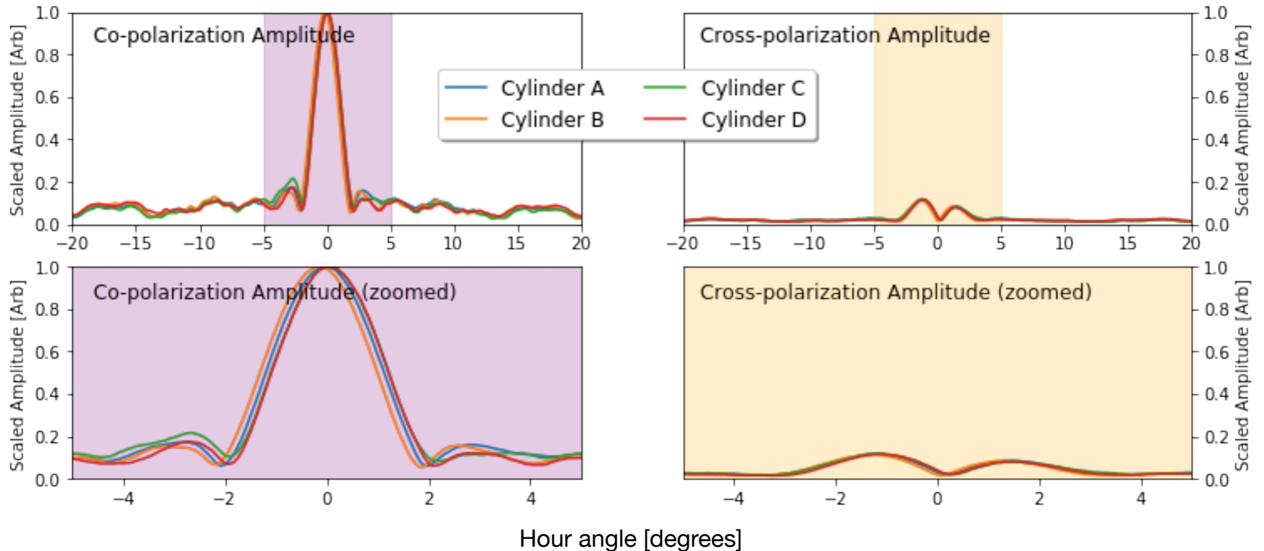
Holographic measurement of a Cyg A transit between the 26m at DRAO (tracking) and CHIME at 717 MHz. Shown is the median amplitude over all Y polarisation feeds on each of the 4 cylinders. Left is co-polar, right is cross-polar. Data is normalized by the peak co-polar response.
