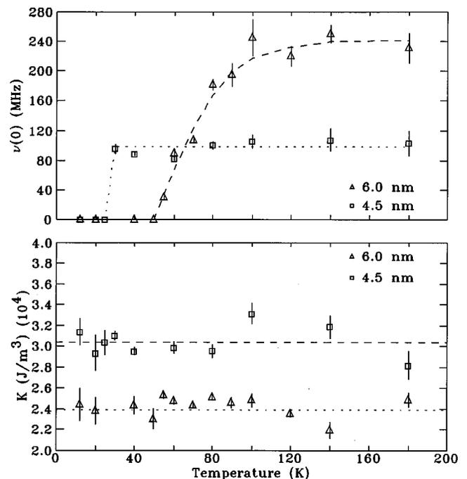
FIG. 2. Plots of the preexponential factor of the relaxation time  $\nu(0)$  and the anisotropy energy  $K$ .  $T_B$  is the point where  $\nu(0) > 0$ .
