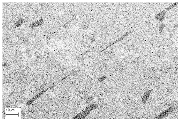
Figure 1. SEM image (back-scattered electron mode, accelerating voltage 20 kV) of the microstructure of \text{EuPdSn} annealed at 600^\circ\text{C} and water quenched (bright phase \text{EuPdSn} ; dark phase, \text{EuPd}_2\text{Sn}_2 ).
