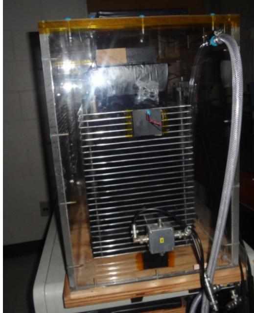
Figure 16: Two of the six piezzo-electric sensors may be seen on one edge of the detector. Also, the tube through which helium enters the chamber is seen on the top right of the chamber.
