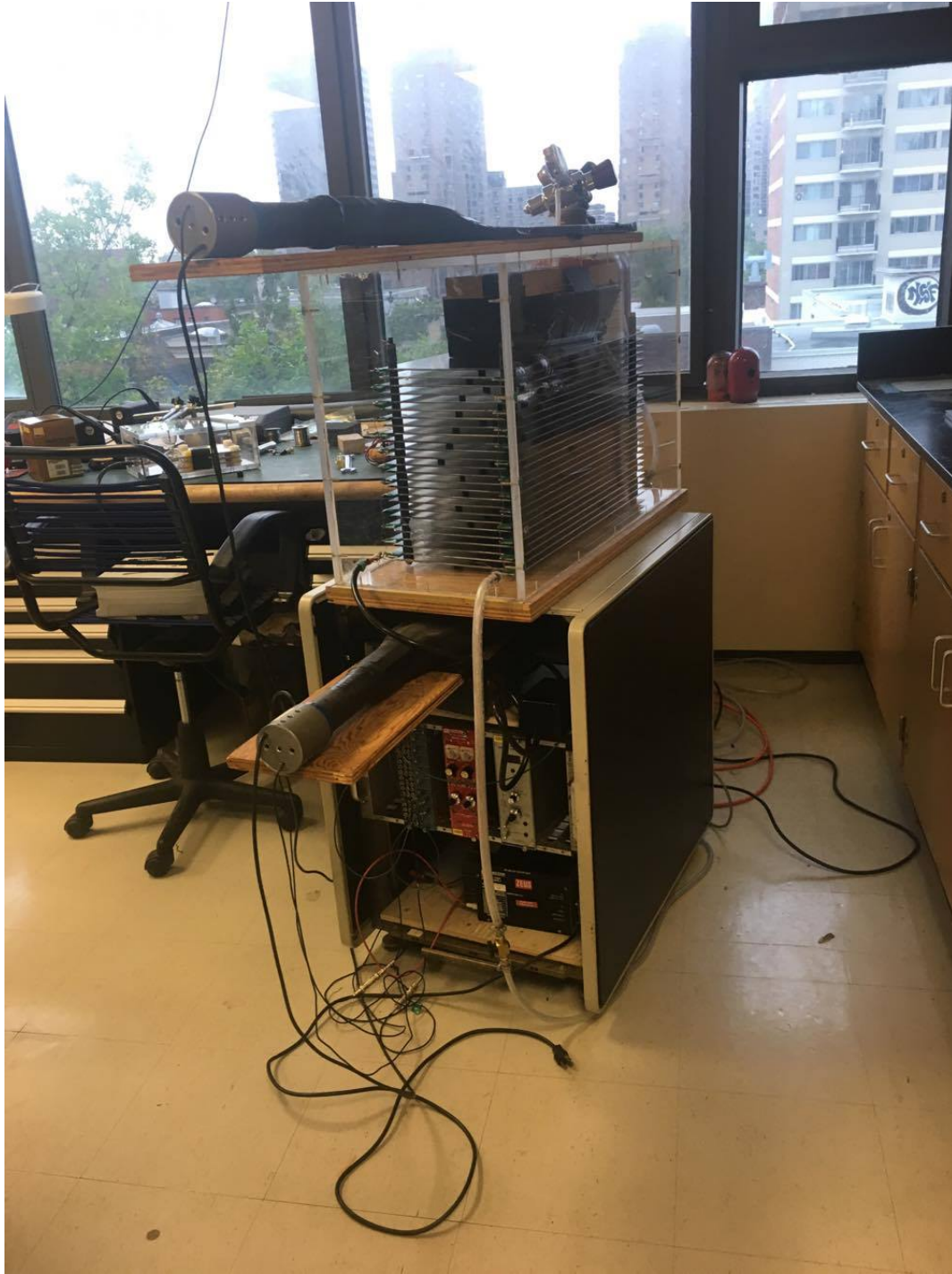
Figure 14: The spark chamber as viewed from one side (the zy -plane). The scintillators coupled with PMT's are above and below the chamber, and the electronics are at the bottom of the cart. The spark chamber is placed near windows as to let helium out of the room.
