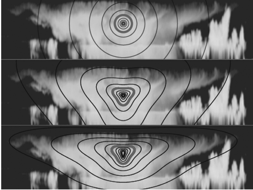
FIGURE 3.4 A CloudSat vertical cloud cross-section with three different scale functions superposed (400 km left to right, 16 km bottom to top; aspect ratio, 6.5:1). The top scale function is isotropic at all scales (circles). In the middle scale function, the rule to change scales is isotropic so that, although the shape of the contours is now anisotropic, it is exactly the same at all scales. The thick gray contour line indicates the (arbitrary) unit scale, and, starting from this, each outer contour is a factor 1.58 enlargement; each inner contour is a factor 1.58 scale reduction. The bottom scale function is the same at the unit scale (thick gray line) as the previous, but now the rule itself is also anisotropic, so that in addition to the 1.58 enlargement, there is also a squashing of factor 1.23 in the vertical. This is the stratification measured for CloudSat vertical sections (Fig. 3.7A). It is close to the theoretical value corresponding to an elliptical dimension of 23/9 .
