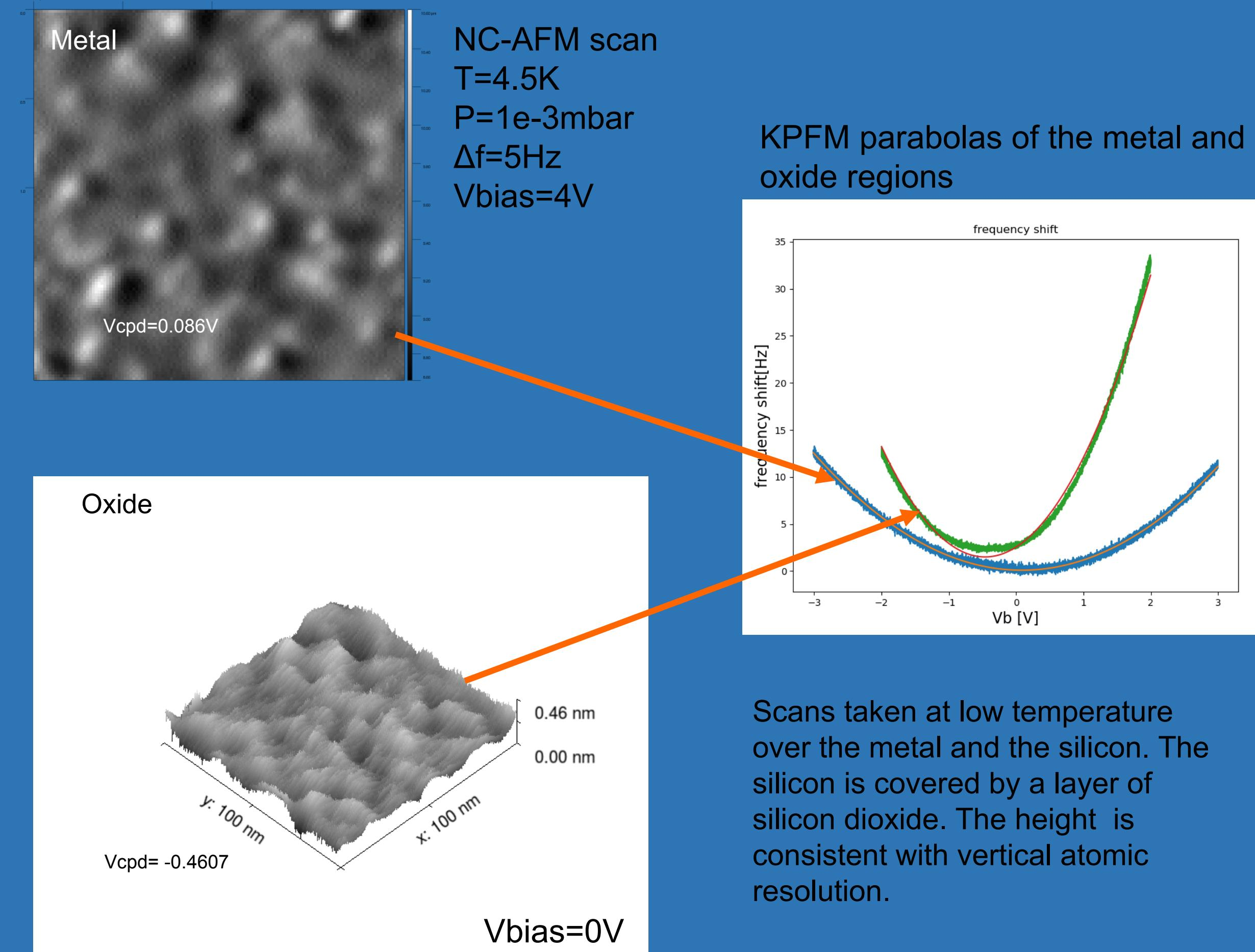
Scans taken at low temperature over the metal and the silicon. The silicon is covered by a layer of silicon dioxide. The height is consistent with vertical atomic resolution.
