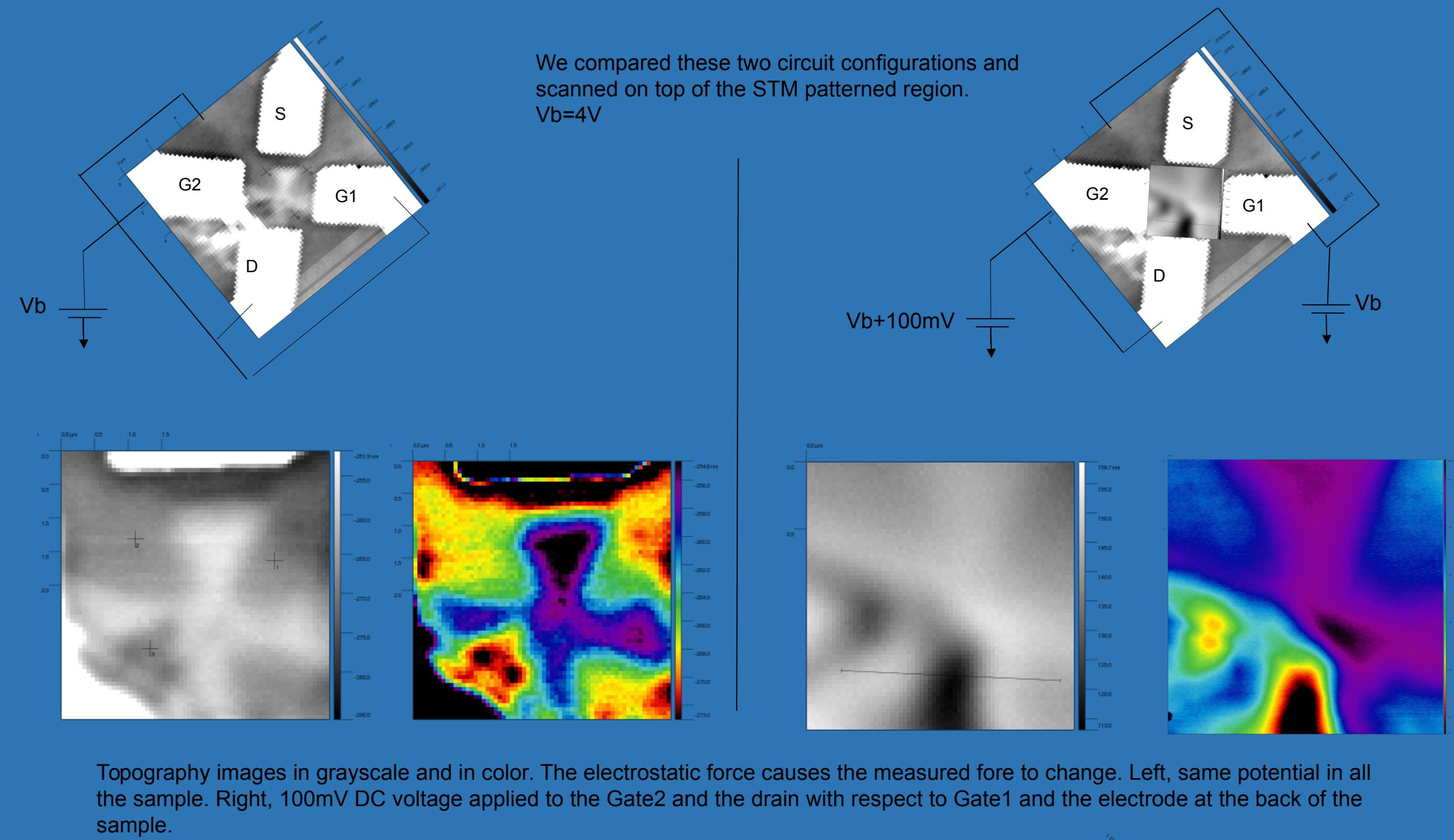
We compared these two circuit configurations and scanned on top of the STM patterned region.
